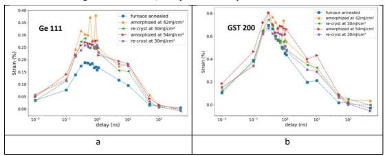
**Fig. 1**: Strain evolution for Ge 111 (a) and GST 200 (b) at various time delays between laser pump and X-ray probe and for 5 different samples. These time-resolved experiments were performed at a fluence of 18 mJ/cm<sup>2</sup> on an initially 50 nm-thick oven-crystallized GGST thin film.
