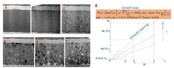
Figure 1: (A-F) Corrected for distortions, bright field defocused cross-sectional TEM images of voids in Si/NGGST/SiN samples annealed at various temperatures and durations; (g) The growth law derived from the mature-state voids characteristics measured after isothermal and isochronal annealing, illustrating the dependence of void size (volume) and density on time and temperature.
