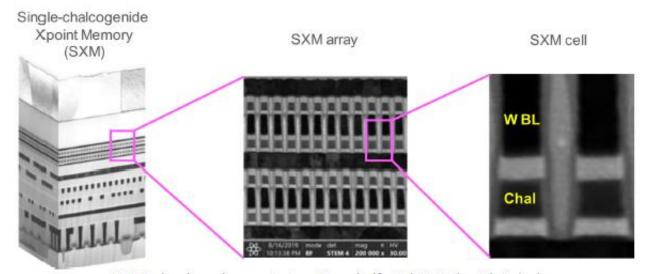
SXM technology demonstrator: 20nm half-pitch 256Gb with 4 decks
