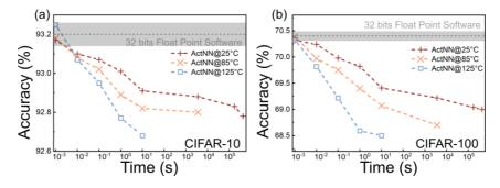
Figure 2 The effect of time and temperature on the inference accuracy of ActNN with (a) CIFAR-10 and (b) CIFAR-100 datasets based on the performance of MLPCM.
