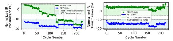
**Figure 1.** Infrared transmission response of a GST/GGSTN stack under repeated irradiation with milliseconds pulses for crystallization and microsecond pulse for amorphization.
