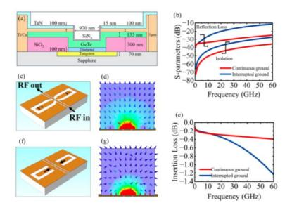
Fig. 1: (a) RF switch cross-section (dimensions not to scale). (b) Reflection Loss & Isolation plot. (c) Interrupted ground plane layout (substrate thickness not to scale) producing (d) bulged E-Field (Transverse to the RF signal propagation). (e) Insertion loss plot. (f) Continuous ground plane (additional ground plane segments shown by the arrows) layout with (g) confined E-Field.
