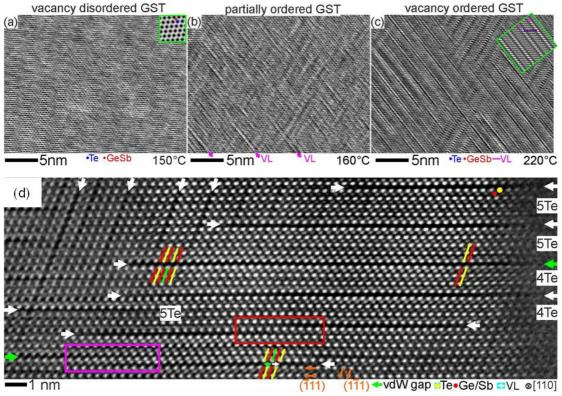
**Fig. 1.** (a), (b) and (c) HRTEM micrographs acquired at TEM holder temperatures of 150°C, 160°C and 220°C, respectively. Insets in (a) and (c) show simulated HRTEM images. VL shows a vacancy layer. (d) HAADF-HRSTEM image acquired after thermal heating of GST225 thin film in TEM to a holder temperature of 240°C. Yellow and red strokes depict Te and GeSb layers, respectively. Green stroke marks the core of transition area and extra Te plane. The rectangles depict layered defects.
