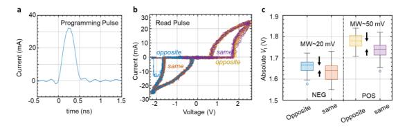
Fig. 2: Electrical characterization of sub-nanosecond programming. (a) Oscilloscope capture of a typical programming pulse with a 300 ps pulse width, 70 ps rise/fall time, and 7.5 V amplitude. (b) Current-voltage (I-V) characteristics measured after  $\sim$ 120 programming pulses. (c) Extracted threshold voltages for positive and negative read operations. Results confirm that the SOM device exhibits a measurable memory window under sub-nanosecond programming conditions.
