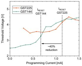
Fig. 1: SET/RESET Threshold Voltage (V<sub>th</sub>) of 1T1S1R devices integrating either GST225 or GST144. The inset shows the device architecture, from top to bottom: Top Electrode (TE), OTS, Intermediate Metal, PCM, Heater element, and Bottom Electrode (BE).
