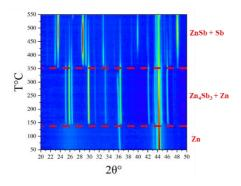
**Fig. 1**: *in situ* XRD recorded during ramp annealing (5°C/min) on a ZnSb cosputtered thin film. The horizontal dotted red lines delimitate temperature domains of each phase.
