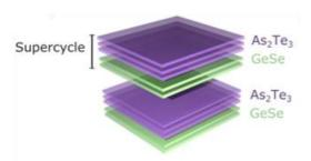
Figure 1: Schematic of the supercycle approach - alternating GeSe to As<sub>2</sub>Te<sub>3</sub> cycles to produce GAST films
