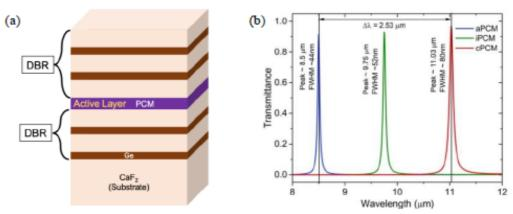
Fig-1: (a) Design of Fabry-Perot filter on CaF2 substrate. (b) Simulated transmittance spectra for amorphous, intermediate, and crystalline phases of GSST41.
