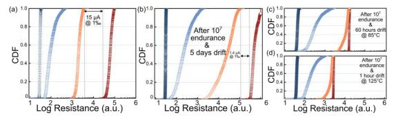
Figure 1 CDFs of the four resistance states of MLPCM cells: (a) fresh device, (b) five days after 10<sup>7</sup> switching cycles, (c) after 10<sup>7</sup> switching cycles followed by 60 hours at 85 °C, and (d) after 10<sup>7</sup> switching cycles followed by 1 hour at 125 °C.
