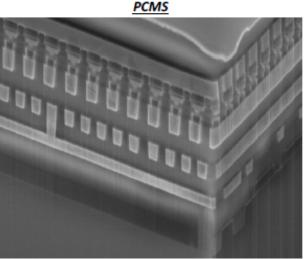
One layer of  $4\lambda^2$  PCMS array stacks on the top of 2level metal CMOS circuits for bitline and wordline select/decode functions.
