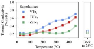
Figure 4 Comparing the different superlattices, it is clear that the choice of TMD has a large effect on the thermal conductivity. especially at high-temperatures.
