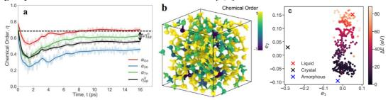
Fig. 1. 200 eV primary knock-on Te atom simulation: a Time evolution of the chemical order within the glassy network of the amorphous  $Ge_2Sb_2Te_5$  model. b Local quasi-binary chemical order in the glassy structure after the event. c 2D SOAP-based similarity map visualizing the entire molecular-dynamics trajectory, plotted as a function of the calculated potential energy of the modelled system, at each point.
