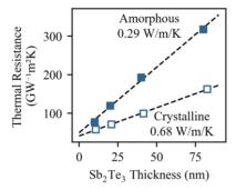
Figure 3 Sb<sub>2</sub>Te<sub>3</sub> by itself shows a high contrast in thermal conductivity between its amorphous and
