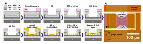
Figure 1. (a) Fabrication flowchart for BEOL integration of ALD PCM on the foundry-processed chips. Most of the photolithography steps are implied. (b) Layout of a 300  $\mu m$  square pixel with heavily doped tapers, and a 40  $\mu m \times 60$   $\mu m$  medium doped region (cyan dashed rectangle) for the PCM metasurface and optical element. The diode selector and presumed off-chip ground and voltage source are also depicted for reference.
