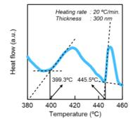
**Fig. 2.** DSC heating curve of V-Te thin film Color modifications from Ref. [3].
