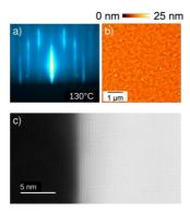
Fig. 1 Structural characterization of the epitaxial Te film deposited on Si(111)–( $\sqrt{3}\times\sqrt{3}$ )R30°–Sb surface at 130°C. (a) RHEED image along a Si(11 $\bar{2}$ ) azimuth. (b) AFM topography image. (c) High-angle annular dark-field STEM micrograph along the [11 $\bar{2}$ 0] zone axis of Te.
