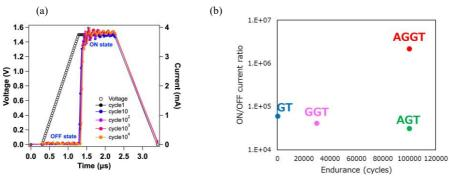
**Fig. 2** (a) Dynamic transient current measurement in the AGGT device. (b) Summary of the ON/OFF current ratios and endurance. The OFF current was  $1.5 \times 10^{-7}$  A,  $3.7 \times 10^{-7}$  A, and  $8.6 \times 10^{-8}$  A for the GT, AGT, and GGT devices, respectively.
