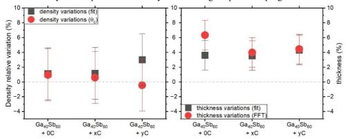
Figure 1: Relative variations between the amorphous and the crystalline phases for the density (left) and film thicknesses (right) obtained from XRR data. Black squares are the results from the simulation and fitting of the full XRR curves, while red circles are extracted from the position of the critical angle (density) and the FFT peaks (thickness).
