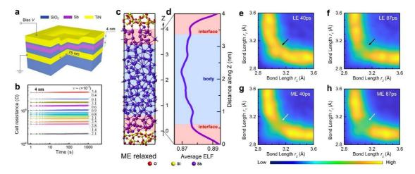
Figure 1. (a) Schematic of the 4 nm-thick Sb-based PCRAM device. (b) Temporal evolution of 12-level resistance states achieved by iterative RESET operations. (c) Amorphous ME model and (d) average ELF value along the thickness Z direction of Sb part. The degree of Peierls distortion evaluated by ALTBC analysis for the 300 K-annealed amorphous LE and ME Sb model at 40 ps (e and g) and 87ps (f and h), respectively.
