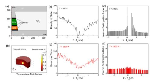
Fig. 1. (a) Model of the OTS+PCM nanodevice used for finite element analysis. (b) Transient temperature distribution in the device during the holding-on stage. Electronic properties of amorphous and liquid GeSe calculated by HSE06 functionals. (c-d) DOS and IPR of amorphous GeSe, respectively. (e-f) DOS and IPR of liquid GeSe, respectively.
