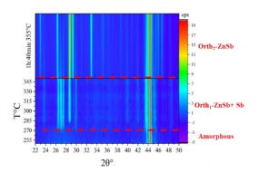
**Fig. 2**: in situ XRD recorded during ramp annealing (5°C/min) from 50 to 350°C followed by an isotherm (1h:40min) on a  $Zn_4Sb_3$  co-sputtered thin film. The horizontal dotted red lines delimitate temperature domains of each phase.
