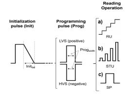
Fig. 2: Schematic of the programming protocol. High (HVS) and Low Voltage State (LVS) are obtained by applying negative and positive Prog pulses, respectively.
