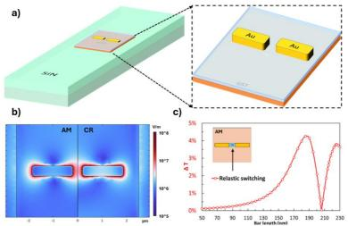
Fig. 1 a) The simplified all-optical plasmonically enhanced cell. A 500 x 500 nm GST patch 10 nm in thickness with a 5 nm thick ITO capping layer is deposited on top of a 1200 x 334 nm Si<sub>3</sub>N<sub>4</sub> waveguide. On top of this are 40 nm wide, 30 nm thick Au bars. b) Normalised E-field distributions for the amorphous and crystalline phases. c) Optical contrast as a function of Au bar length, assuming realistic phase switching.
