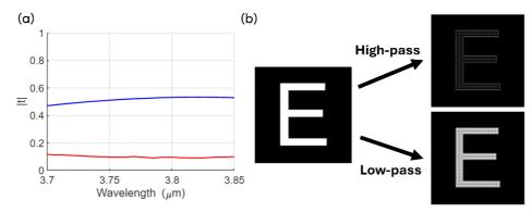
Fig. 2 (a) Experimental transmission results of the higher amorphous phase (blue line) and the near-zero crystalline phase (red line) around the crystalline minima ( $\sim 3.8 \mu m$ ). (b) Functionality simulation results using the experimental results to show high-pass filtering (top) and low-pass filtering (bottom).
