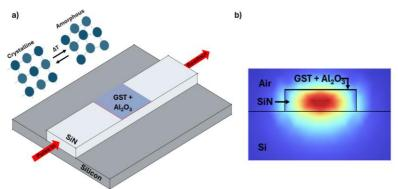
Fig. 1 a) Schematic of a 'conventional' integrated photonic phase-change memory device. A 10 nm GST layer with a 5 nm Al<sub>2</sub>O<sub>3</sub> capping is fabricated on top of a Si<sub>3</sub>N<sub>4</sub> waveguide 1.2 μm in width and 334 nm high. b) Simulated cross-section of the waveguide in operation showing the TE mode which couples evanescently to the GST cell.
