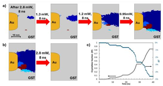
Fig. 2 a) Evolution of the GST phase distribution as a succession of crystallising optical pulses is applied. b) Change in GST phase distribution as a re-amorphising pulse is applied. Regions of colour represent crystallite grains of different orientations. c) Evolution of GST crystalline fraction in a 50 x 50 nm region centralised between the Au bars and the readout contrast both during the crystallisation shown in a).
