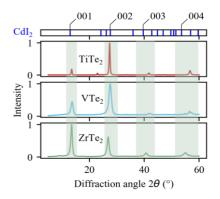
Figure 2 Ex-situ XRD after a 400°C anneal shows that all three materials form the CdI<sub>2</sub> structure with 00L planes parallel to the substrate.
