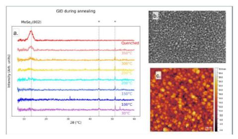
Fig. 1 Characterization of MoSe<sub>2</sub> thin films: (a) GID scans collected during annealing, showing the emergence of the (002) diffraction peak around 250 °C, indicating the onset of crystallization; (b) SEM image of an as-deposited ~80 nm thick film, revealing a fine-grained, uniform surface morphology without visible defects or cracks; (c) AFM image of the same as-deposited film, confirming homogeneous surface coverage and consistent nanoscale features observed by SEM.
