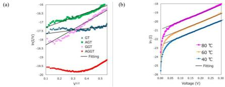
**Fig. 3** (a) The ln(I/V) as a function of  $V^{1/2}$  for verifying the Poole–Frenkel conduction. (b) The ln(I) as a function of V for verifying the Schottky conduction in the AGGT device.
