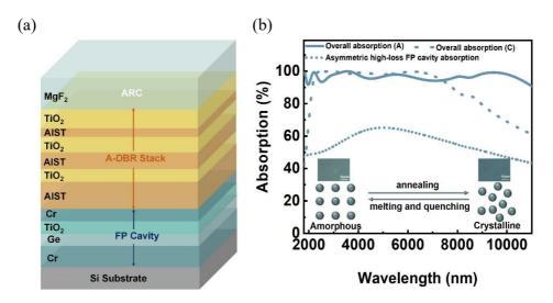
**Figure 1.** Schematic and optical response of the proposed absorber. (a) Schematic illustration of the ultrabroadband absorber architecture. (b) Simulated absorption spectra of the integrated structure before and after phase transition, along with the optical response of the Fabry–Pérot cavity. The insets depict the experimentally observed phase transition behavior.
