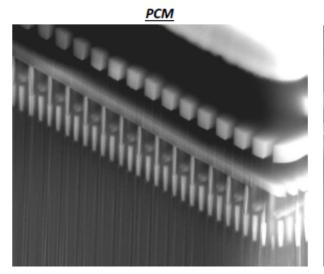
8λ<sup>2</sup> BiPCM array with a CMOS based circuits for bitline/wordline select/decode functions, not shown, are implemented at the edge of array.
