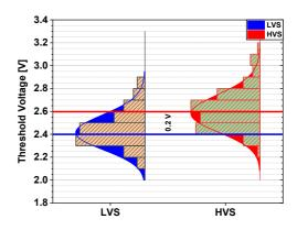
Fig. 3 Impact of readout technique on the memory window (MW). The SP method results in the widest MW along with reduced variability. Data points indicate the average MW, while the solid lines represent the corresponding standard deviation.
