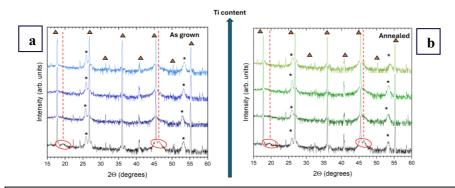
Figure 1: a,b) Diffraction curves of Ti-doped GST samples. Peaks marked with orange triangles are related to Mica substrate. Reflections marked with black asterisks refer to cubic GST phase. The vacancy layers peaks (red circles) disappears when Ti is added.
