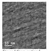
Figure 1 Cross-sectional TEM image of a sputtered superlattice with a period of 5 nm Sb<sub>2</sub>Te<sub>3</sub> and 3 nm TiTe<sub>2</sub>.
