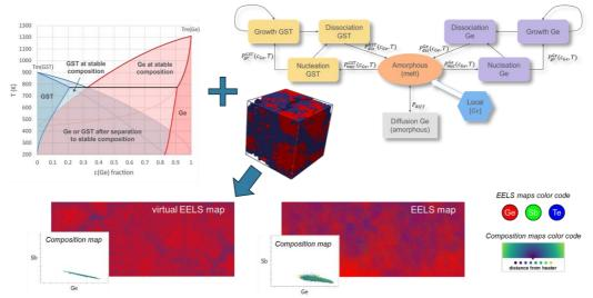
Figure 1 – The framework for simulating the BEOL anneal relies on the eutectic decomposition of Ge and GST domains and on a KMC algorithm derived from a stochastic model of crystallization. (Bottom) Virtual EELS and composition maps obtained with simulations compared to experimental outcomes.
