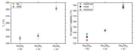
Figure 2: Left: the crystallization temperatures obtained for the 3 samples extracted starting from the sheet resistance (Rs) and for in-situ XRD (XRD). Right: the 10-year crystallization temperature obtained from extrapolating the Arrhenius equation linking the incubation time and the temperature of several isotherms. The graph shows the shortest (minimum), the average + standard deviation (mean) and the longest (maximum) extrapolated time.
