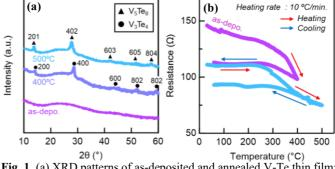
Fig. 1. (a) XRD patterns of as-deposited and annealed V-Te thin film; (b) temperature dependent resistance of V-Te thin film Color modifications from Ref. [3].
