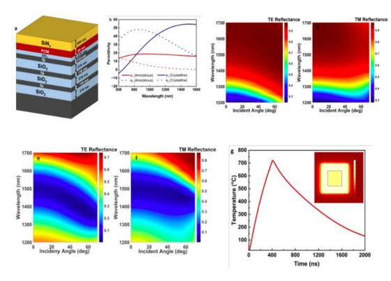
Fig1: (a) The optical modulator design, (b) measured dielectric permittivity of the Ge-rich Ge-Sb-Te phase change material, (c) & (d) amorphous phase reflectance over various incident angles and wavelength for TE and TM polarisations, (e) & (f) crystalline phase reflectance over various incident angles and wavelength for TE and TM polarisations, (g) electro-thermal simulations for amorphization.
