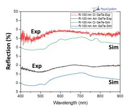
**Fig.2**: Experimental and simulated reflection of a combined silica-GeTe metasurface prepared by "NIL as a mask approach".
