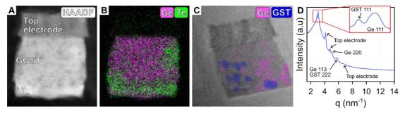
**Fig. 1** (A) STEM-HAADF image of a representative GGST cell with (B) its elemental map showing Ge, Sb and Te after a thermal pulse at 380°C. (C) HRTEM image of another GGST cell heated at 400°C, showing evidence of Ge and GST cubic phases inside the cell. (D) Radial integration profile of the corresponding FFT of (C) used to identify the different phases.
