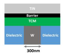
Fig. 1: Simplified schematic of the analytical TCM GSSN 1R device.
