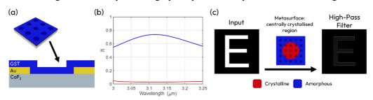
**Fig. 1** (a) A schematic of the EOT device design. (b) Simulated transmission response of the device in the mid-infrared for the amorphous (blue line) and crystalline (red line) phases. (c) Simulated high-pass filter functionality of a device design functional in the mid-infrared.
