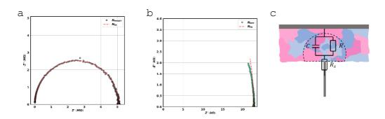
Figure 1 – a) Nyquist plot of the RESET state. b) Nyquist plot of the SET state. c) Schematic drawing of the equivalent circuit.
