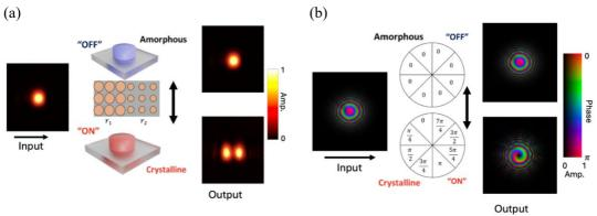
**Figure 1:** (a) Schematic and experimental results of a switchable phase-change metasurface performing  $ON/OFF\ TEM_{00}$  to  $HG_{10}$  mode conversion. (b) Schematic and simulated performance of a switchable metasurface for ON/OFF optical orbital angular momentum control.
