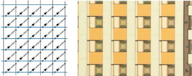
Figure 2. (Left) Circuit diagram of the cross-bar matrix heater array with selector for preventing sneak path current. (Right) Top-view optical micrograph of the 2-D micro-heater array.
