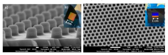
Fig. 1: (a) SEM images and (b) photos of GeTe metasurface fabricated via the etching strategy; (c) SEM images and (d) photos of GeTe metasurface produced by the template strategy. Both samples were produced on  $1 \times 1$  cm<sup>2</sup>.
