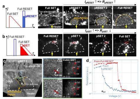
Fig. 1: Pulse squences (on the left) and TEM DF images (on the right) of IRSs in G-GST cells accessed by (a) partial amorphization of the dome intially in the crystallized Full SET state, and (b) partial crystallization of the dome initially in the amorphous Full RESET state. (c) TEM HR images of a partially crystallized dome created by pSET. (d) Resistance as a function of pSET voltage when starting from the Full RESET or from the pRESET state.
