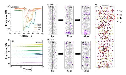
**Fig. 1** (a) The R-V electrical test of the PCM cell using GST-C. (b) The resistance drift coefficient  $\nu$  of the GST-C phase-change cell obtained by fitting with the equation. The evolution of the crystallinity of the GST(c) and GST-C(d) models during the first 60 ps of the crystallization process. The ordered cubic local motifs are highlighted in purple. (e) the snapshot of the GST-C system at 60 ps. The primary forms of carbon atom presence are marked with red circles.
