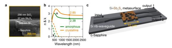
Figure 1 a) SEM micrograph of r-Sapphire-Si-Sb<sub>2</sub>S<sub>3</sub>-SiO<sub>2</sub> multilayer cross-section with listed thicknesses. b) Measured refractive index and absorption coefficient of 37 nm Sb<sub>2</sub>S<sub>3</sub> film from (a) in amorphous (green) and crystalline (orange) phases. The dashed line highlights the 1550 nm wavelength of interest. c) Scheme of the inverse-designed Si- Sb<sub>2</sub>S<sub>3</sub> tunable integrated meta-switch.
