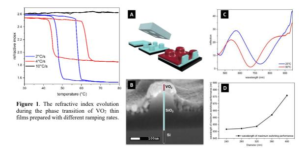
**Figure 2**. Characterization of the conformal metasurface. (A) fabrication schematic, (B) SEM image, (C) reflection spectra, and (D) relationship between pillar size and maximum switching wavelength.
