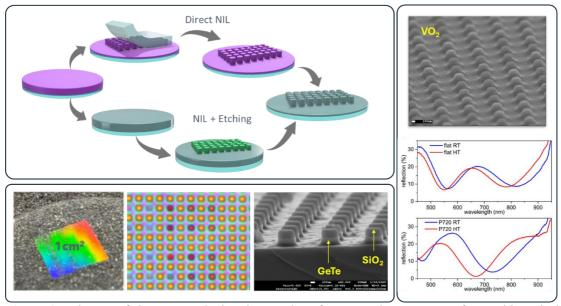
Figure 1. Schemes of the NIL method and examples of GeTe and VO<sub>2</sub> metasurfaces with optical switching capability.
