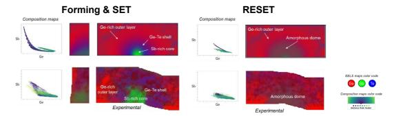
Figure 2 – EELS and composition maps for forming/SET pulses and for RESET pulses, obtained with simulations (top) and experimental data (bottom). All the main regions are correctly identified by the simulation.
